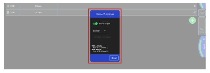
In this options window you can enable sound to light for this chase. You can also set the "Energy" option to look for specific audio frequencies. If this option is left as Energy, it will use the entire frequency spectrum.
