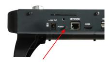
To power up the console, simply plug in the supplied 12v DC power supply. If the console has been shut down via the software, press the power switch on the back panel. After a few seconds the screen will come to life, you will see the operating system loading.
