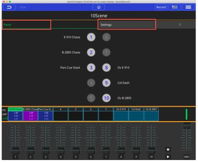
Just like the actual 10 scene wall plates or the 10 buttons on the front panel of the QuickQ Rack, it can be used to trigger **EITHER** the first 10 execute buttons on the execute page or the 10 Playbacks. Choose the option you want in the 10scene settings tab.
