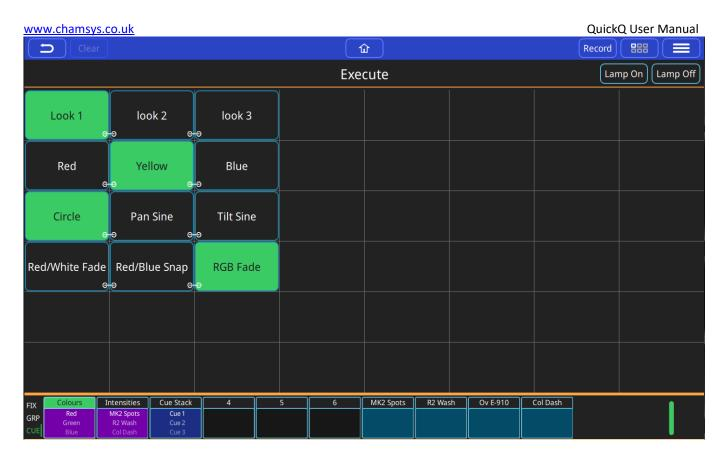
Using the 'link' option will allow for clicking on an execute to release any other executes that are 'linked' to it. In order to Link executes, they must be directly next to each other horizontally. Use the Action Menu to link and unlink execute Items.
