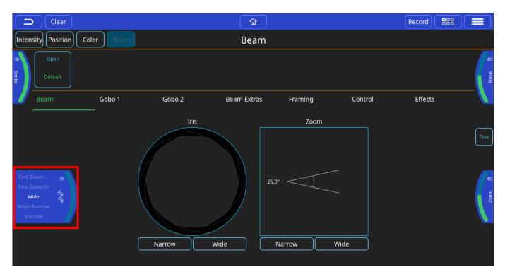
Alternatively a long press and hold on the encoder tab will show selection boxes for those ranges for any given encoder.
